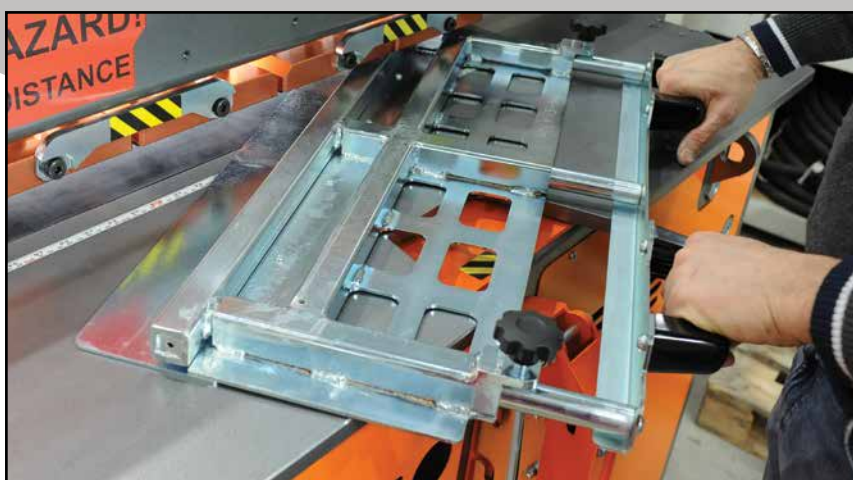
Horizontal positioning frame
