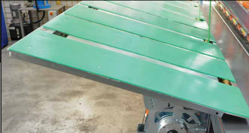
Flat slides for sheets thicker than 15 mm
