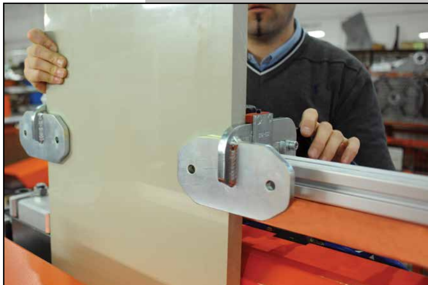
Vertical positioning and fixing for the sheet
