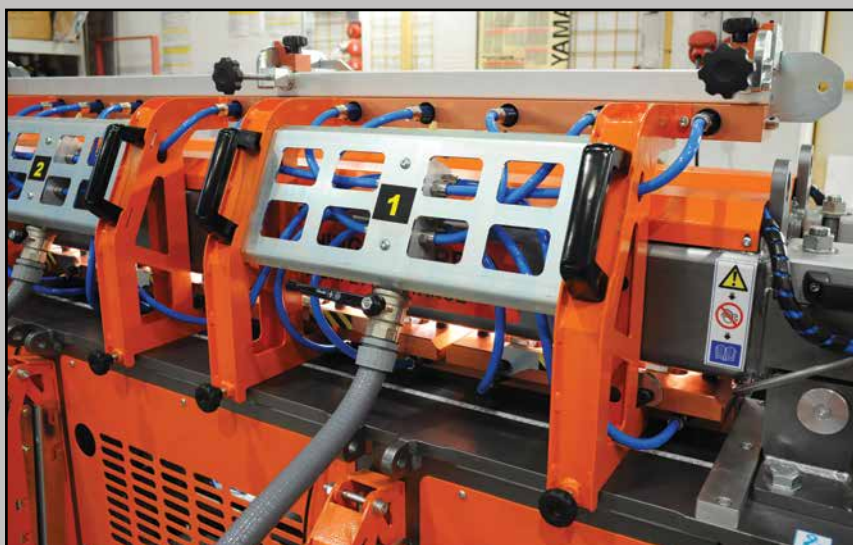
Vacuum system for vertical sheet support
