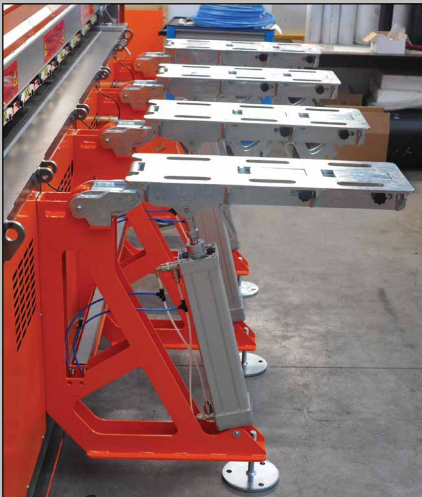
Pushing device works also as lateral supports
