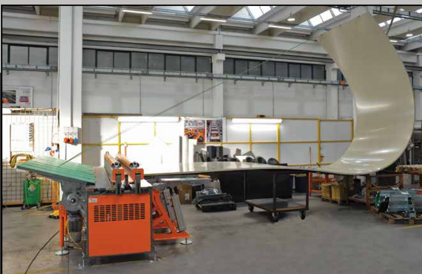
Pulling belts in action
