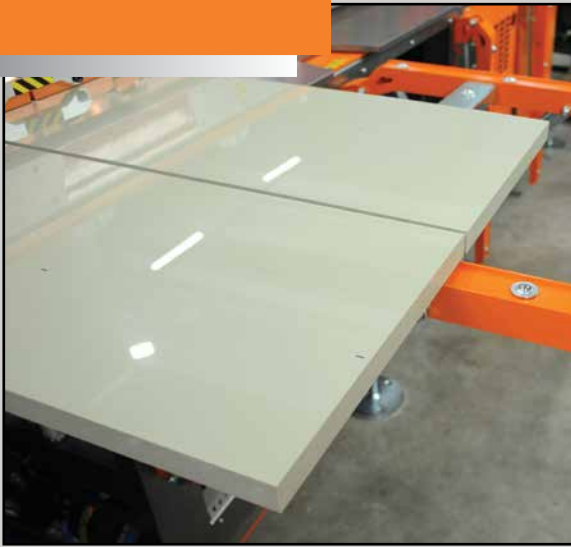
Folding lateral supports with bearing balls for easy sheet movements
